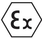
**ATEX II2G Ex h IIC T6 Gb X - II2D Ex h IIIC T85° Db X      -10°C ≤ Ta ≤ +60°C**
